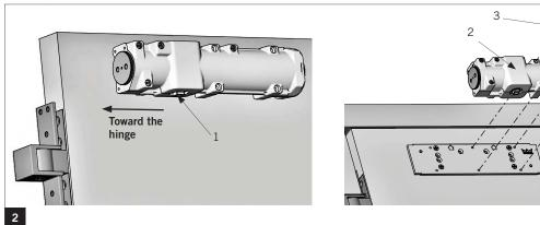
NOTE: Orient pinion (1) closest to hinge.
