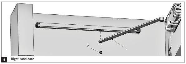
**4.1** Align the arm (1) with the slide shoe of the track channel.
